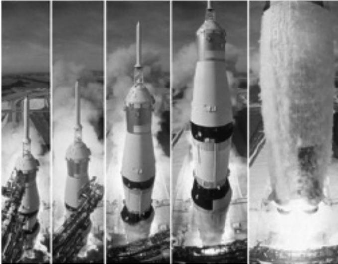
Because rockets take off vertically, they are still attached to the pad to provide stability for several seconds after engine ignition.<sup>64</sup> Once the engines have built up to their full-thrust capacity, the launch pad's connections to the rocket, either through hold-down arms or explosive bolts, are released.<sup>65</sup> Subsequently, the rocket may lift off, free from support or restraint from the launch pad.<sup>66</sup>
